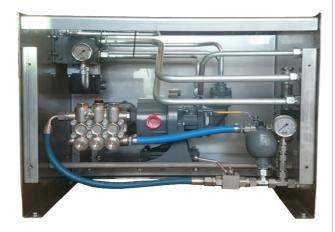
This hydraulic high pressure washer includes one high pressure water pumps which delivers 40l/min at 140 bar. Piping and cabinet is made of stainless steel. Seethrough splash guard in front.
